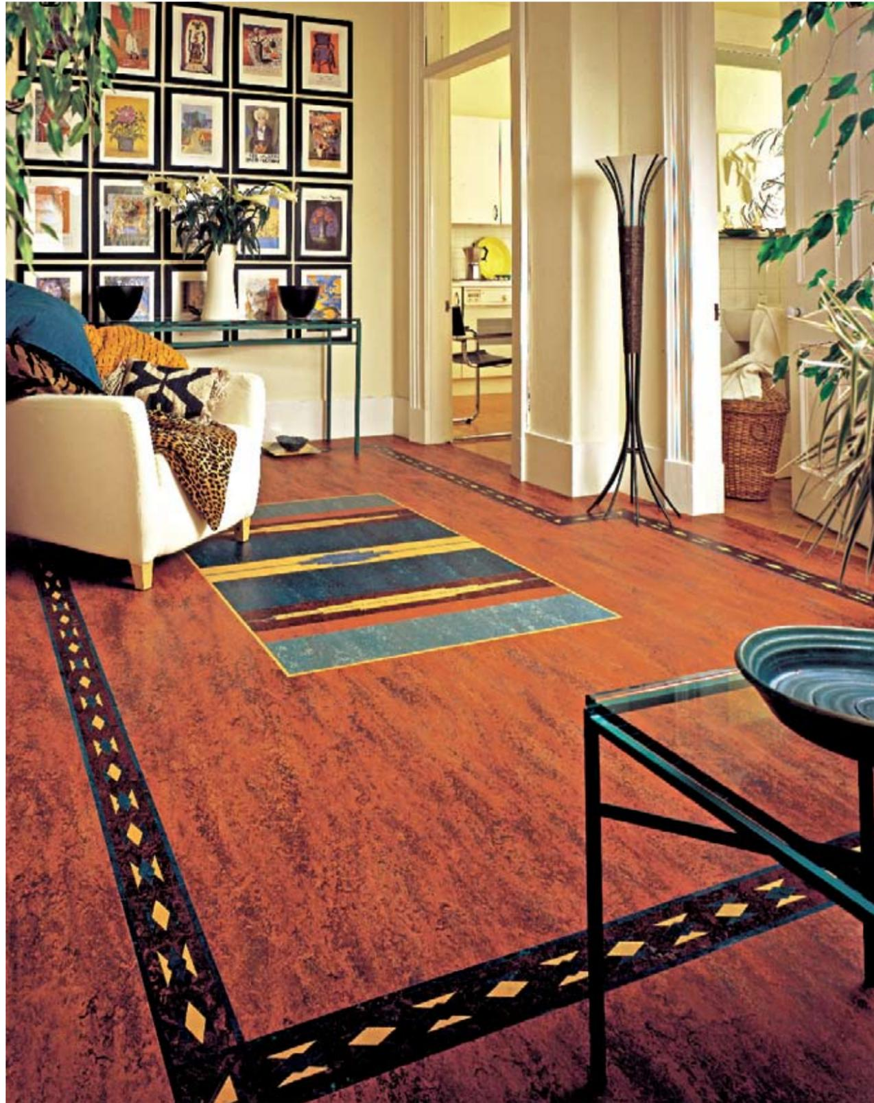
**Linoleum floors with custom designs**, like this one, are especially sensitive to uneven surfaces or debris underneath. Even after it's in place, linoleum is not trouble-free. It can be cleaned with a variety of floor care products, but never with anything containing ammonia.
